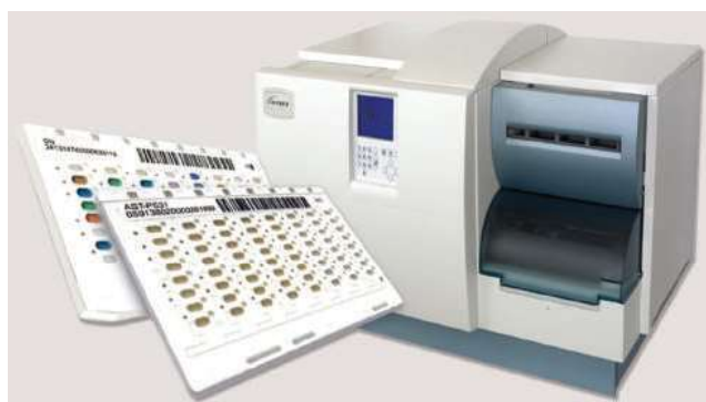
Fig. 3.3.23: VITEK 2 system with its panels (reagent cards) for identification and antimicrobial susceptibility test.
